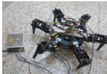
Figure (2): BH3-R hexapod robot of proposed method
