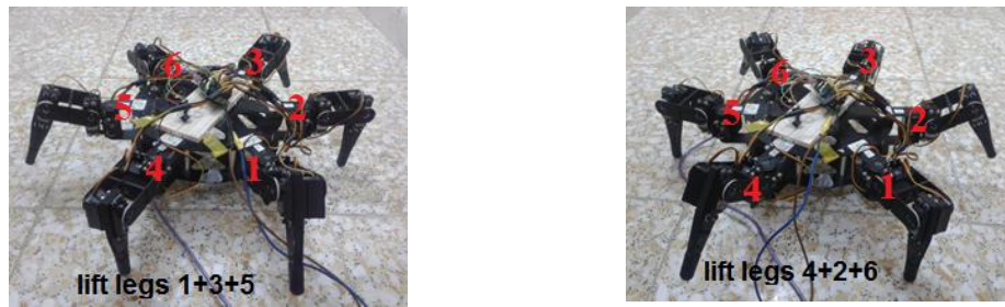
Figure (5): Results of practical real BH3-R hexapod robot sequences for tripod gait
